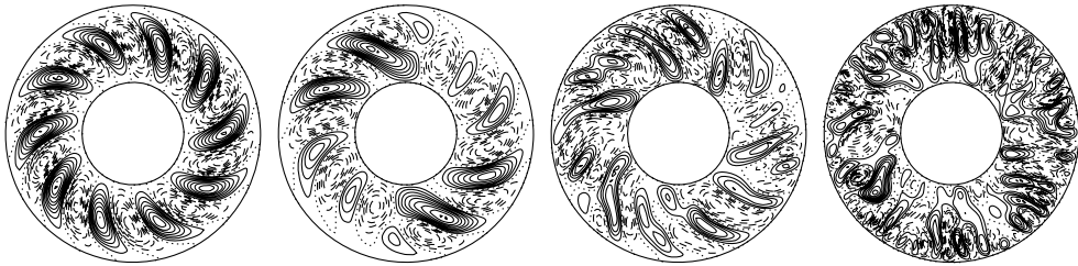
FIGURE 3. Equatorial streamlines r\partial_\phi v = \text{const.} in the case P = 20 , \tau = 5 \times 10^3 and R = 1.6 \times 10^5 , 1.75 \times 10^5 , 2.5 \times 10^5 , 1.5 \times 10^6 (from left to right).
